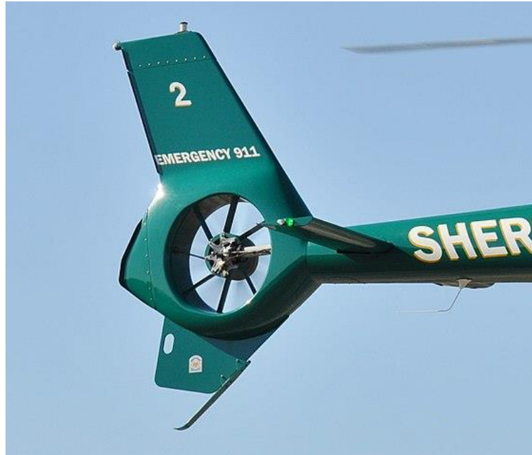
The fenestron anti-torque tail rotor
