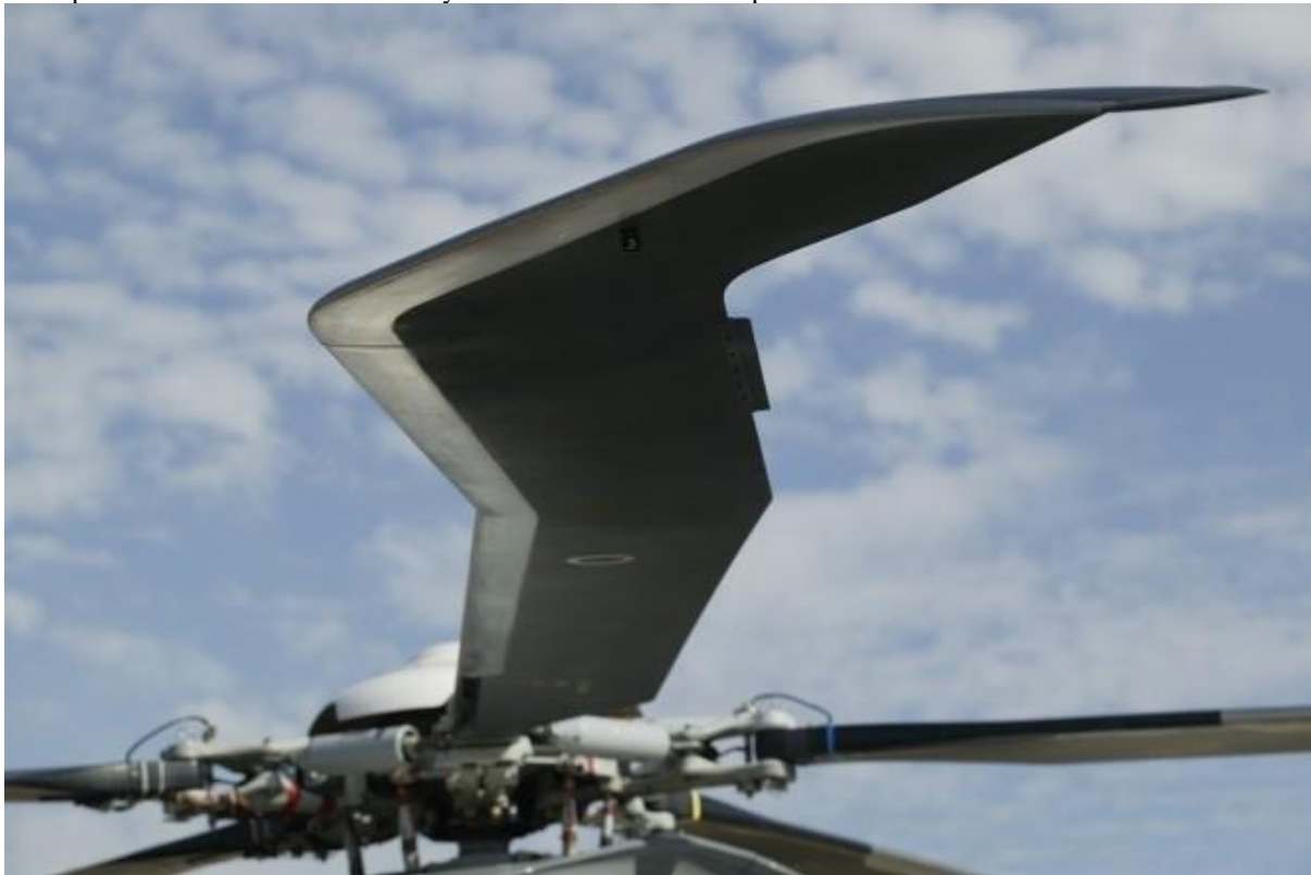
BlueEdge helicopter blades have a unique shape which minimizes blade vortices.
