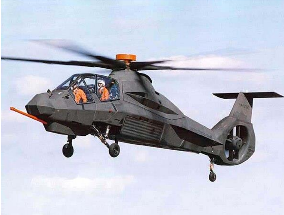
The first RAH-66 Comanche prototype which was a stealth helicopter with an reduced acoustic signature
